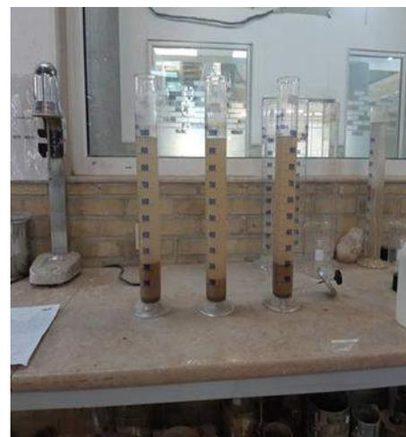
Figure 3. Particle size distribution (hydrometer analysis)
