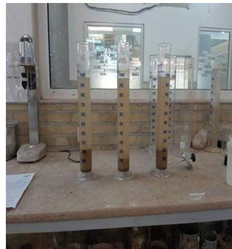
Figure 3. Particle size distribution (hydrometer analysis)
