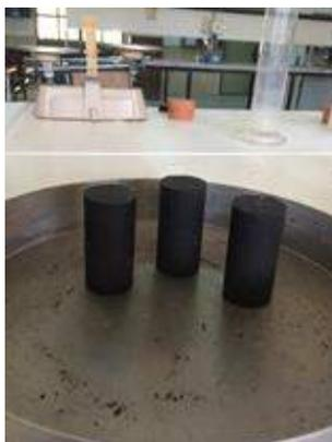
Figure 3. Cylindrical specimen made of organic soil
