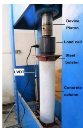
Figure 5. Test setup and instrumentation
