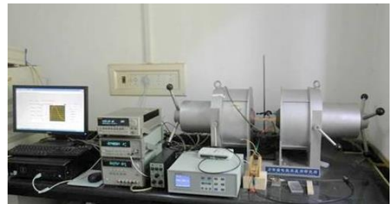
Figure 4. Piezoelectric micro-vibration energy harvester physical map
