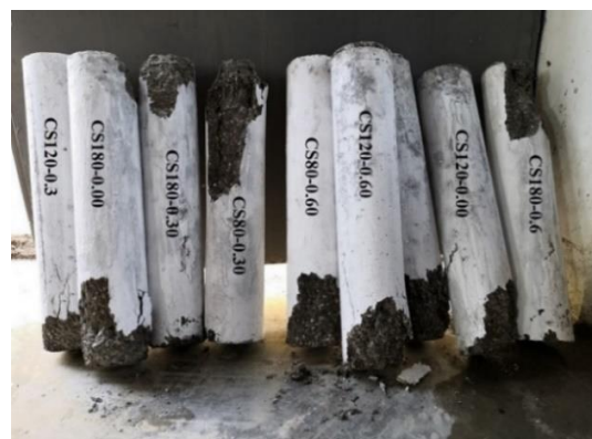
Figure 10. Failure patterns of short columns
