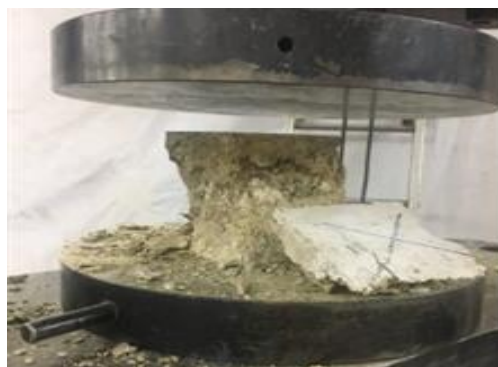
Figure 3. Failure sample of geopolymer concrete
