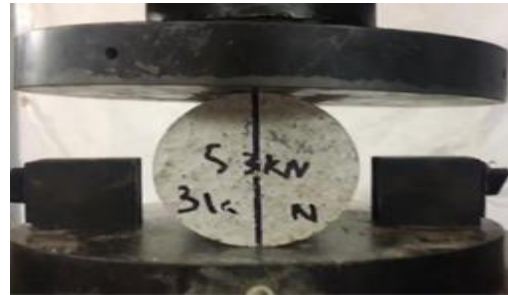
Figure 4. Failure sample of geopolymer concrete
