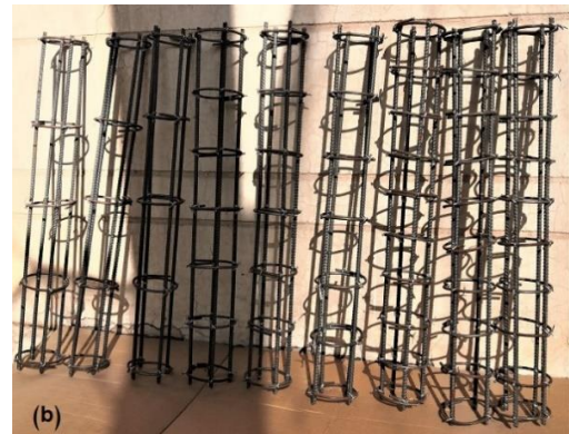
Figure 2. (a) Details of columns showing the spacing between the ties (b) Rebar configuration
