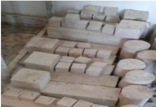
Figure 2. Tensile, flexural, and compression samples made
