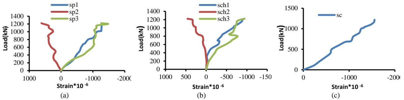
**Figure 17.** Applied load versus steel and concrete strains for composite wall with compressive strength 39MPa and thickness 70mm (a) strain in steel plates (b) strain in steel channel (c) strain in concrete
