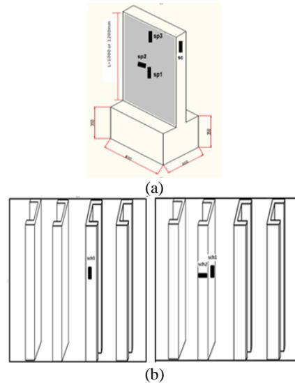
Figure 4. Location of strain gages on (a) steel plate (b) steel channel
