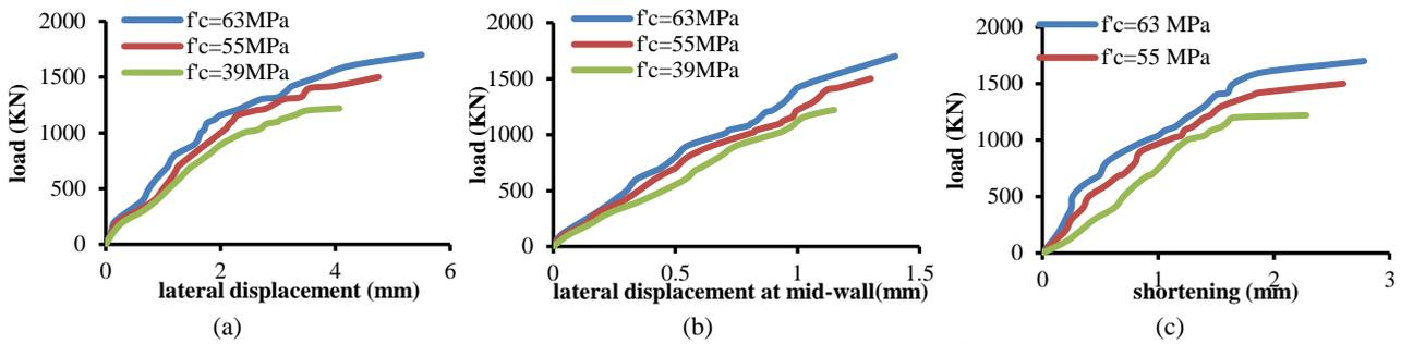
**Figure 10.** Results of the second group (a) load versus lateral displacement at the top height of the wall (b) load versus lateral displacement at mid-wall (c) load versus axial shortening
