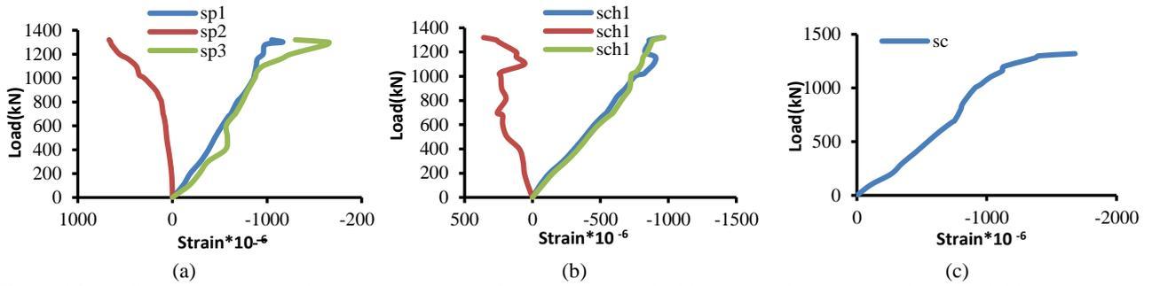
**Figure 16.** Applied load versus steel and concrete strains for composite wall with compressive strength 63MPa and thickness 55mm (a) strain in steel plates (b) strain in steel channel (c) strain in concrete
