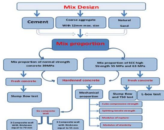
**Figure 1.** Schematic representation of the experimental program
