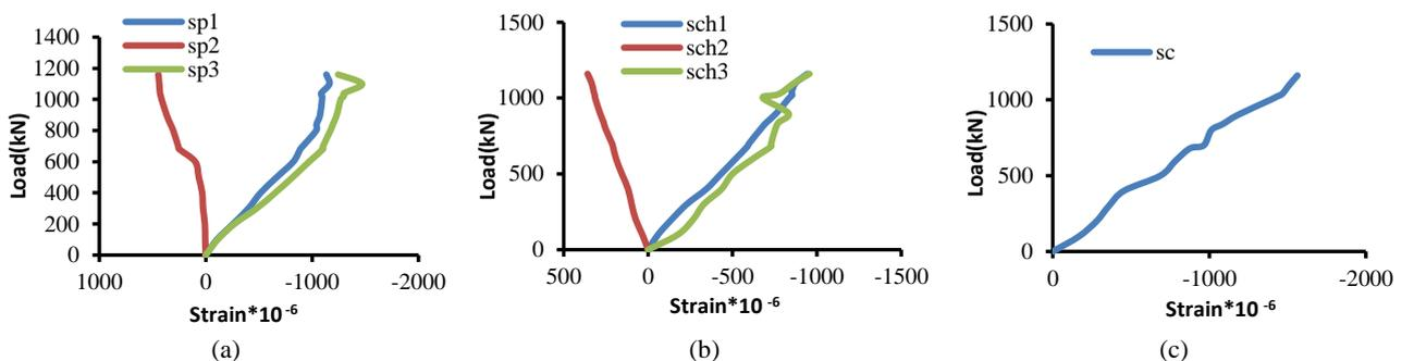
**Figure 15.** Applied load versus steel and concrete strains for composite wall with compressive strength 55MPa and thickness 55mm (a) strain in steel plates (b) strain in steel channel (c) strain in concrete
