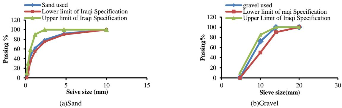
Figure 3. Grading curves for materials
