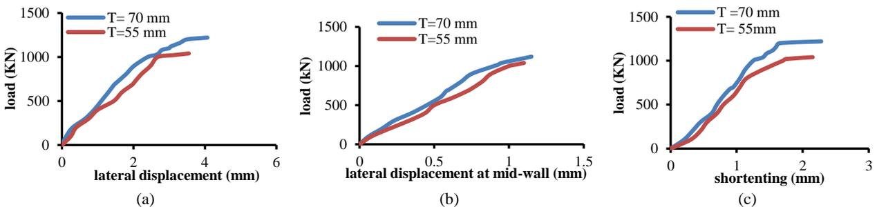
**Figure 11.** Comparison at compressive strength equal to 39MPa (a) load versus lateral displacement at the top height of the wall (b) at mid-height of the wall (c) load versus shortening
