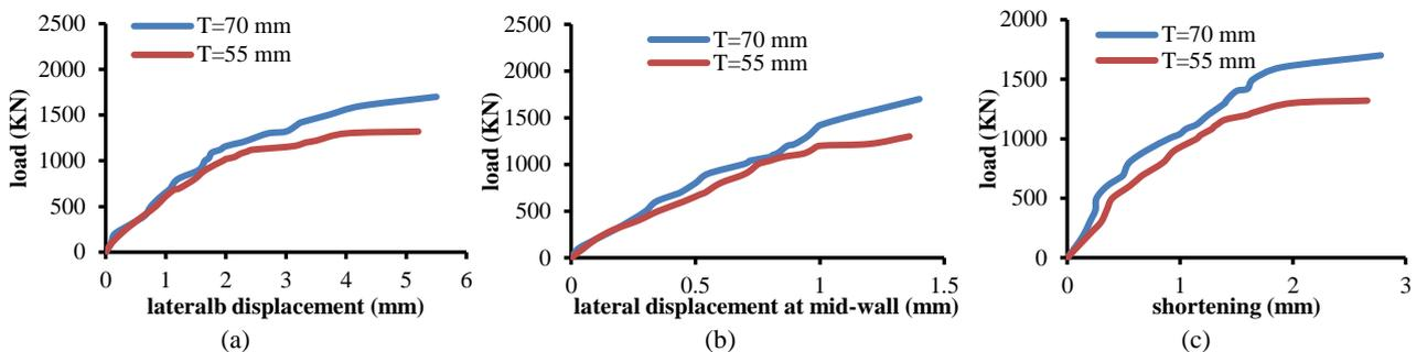
**Figure 13.** Comparison at compressive strength equal to 63MPa (a) load versus lateral displacement at the top height of the wall (b) at mid-height of the wall (c) load versus shortening
