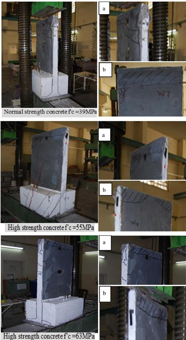
**Figure 8.** The failure mode of the tested walls (group2), (a) Right side, (b) Left side
