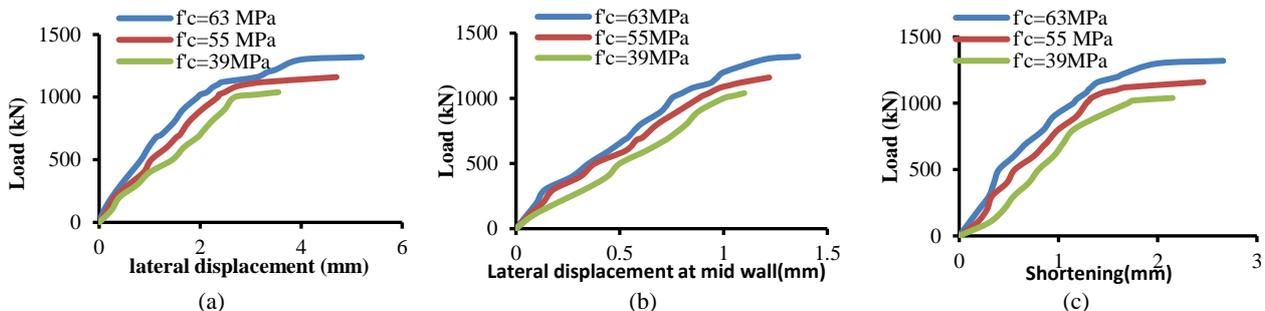
**Figure 9.** Results of the first group (a) load versus lateral displacement at the top height of the wall (b) load versus lateral displacement at mid-wall (c) load versus axial shortening
