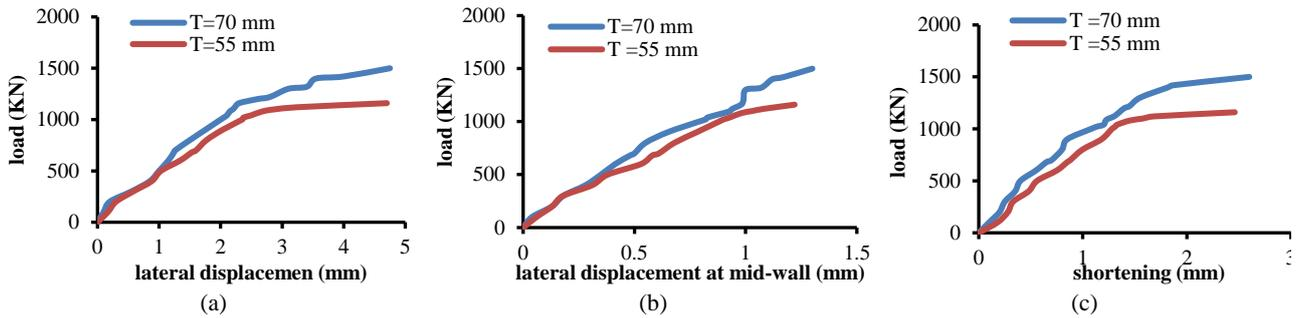
**Figure 12.** Comparison at compressive strength equal to 55MPa (a) load versus lateral displacement at the top height of the wall (b) at mid-height of the wall (c) load versus shortening
