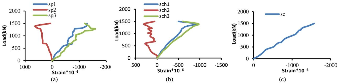
**Figure 18.** Applied load versus steel and concrete strains for composite wall with compressive strength 55MPa and thickness 70mm (a) strain in steel plates (b) strain in steel channel (c) strain in concrete
