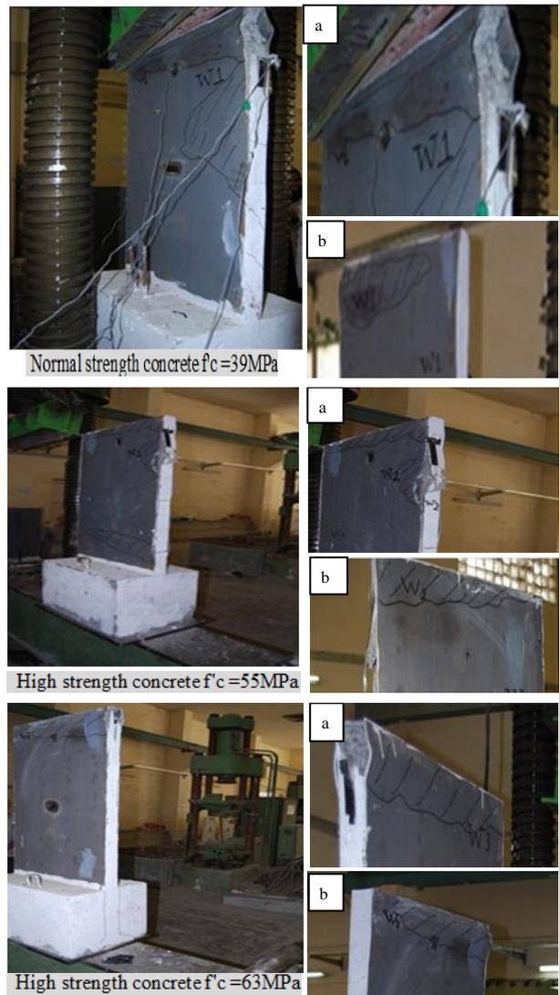
**Figure 7.** The failure mode of the tested walls (group1), (a) Right side, (b)Left side
