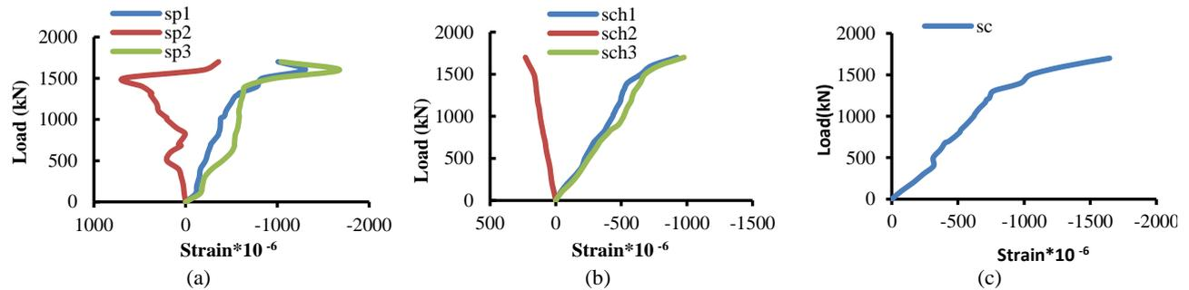
**Figure 19.** Applied load versus steel and concrete strains for composite wall with compressive strength 63MPa and thickness 70mm (a) strain in steel plates (b) strain in steel channel (c) strain in concrete
