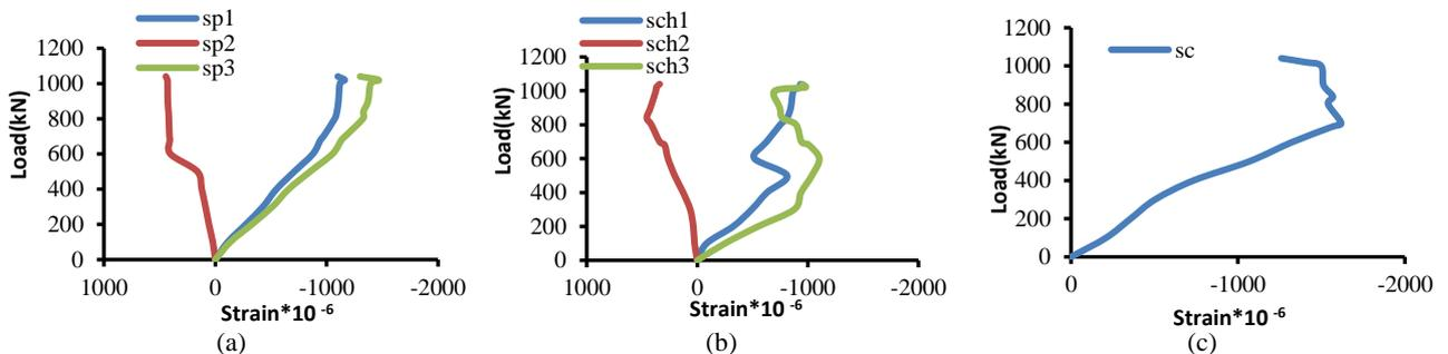
**Figure 14.** Applied load versus steel and concrete strains for composite wall with compressive strength 39MPa and thickness 55mm (a) strain in steel plates (b) strain in steel channel (c) strain in concrete
