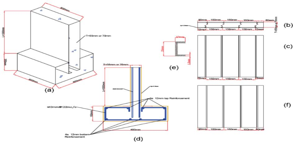
**Figure 2.** Details of all groups (a) isometric view of wall (b) top of the wall (c) right plate with steel channel (d) section through all wall (e) dimension of steel channel (f) left plate with steel channel
