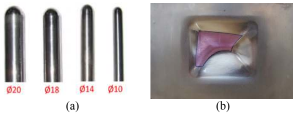
Figure 3. (a) Tungsten Carbide hemispherical forming tools used in the forming process of the mild steel sheets (mm); (b) Final fender of the NP01 formed on the low-carbon steel sheet
