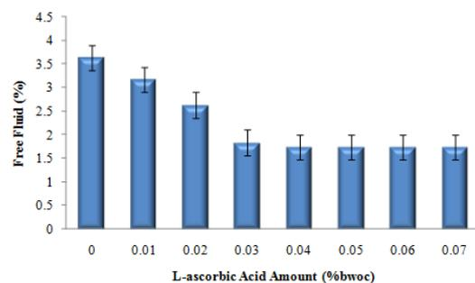
**Figure 2.** Effect of L-AA in different amounts on the free fluid content of cement slurry at 52°C
