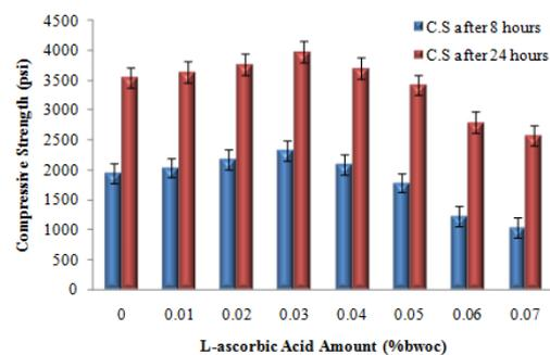
**Figure 5.** Compressive Strength for 8 and 24 hours vs. amount of L-AA used in slurries at 60°C
