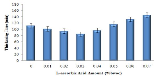
**Figure 4.** Thickening Time vs. amount of L-AA used in slurries at 52°C & 5160 psi
