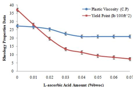
**Figure 3.** Effect of L-AA in different amounts on the rheology properties of cement slurry at 52°C
