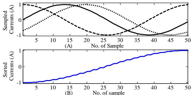
**Figure 13.** (A) Three examples of sampled one-cycle data windows, (B) Obtained waveform after sorting
