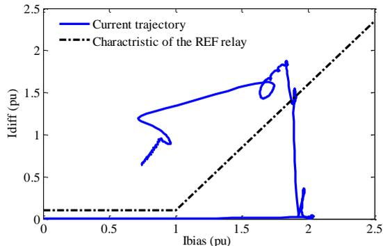
**Figure 11.** Current trajectory based on the modeled REF relay during transformer energization with CT saturation
