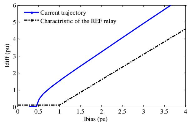
**Figure 5.** Current trajectory based on the modeled REF relay during internal fault
