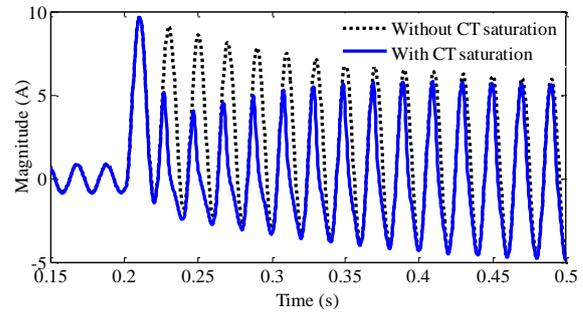
Figure 6. The current of phase A for three phase external fault
