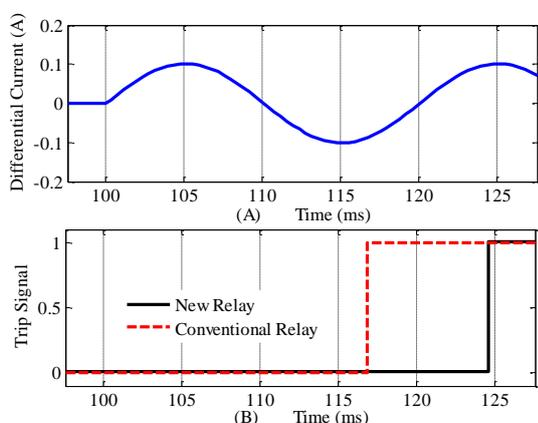
**Figure 16.** (A) Differential current during light internal fault, (B) trip signals
