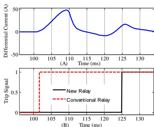
**Figure 15.** (A) Differential current during severe internal fault, (B) trip signals
