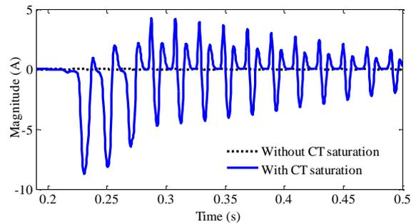
Figure 7. Differential current during external three-phase fault
