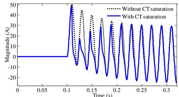
**Figure 4.** Differential current during internal fault with and without CT saturation
