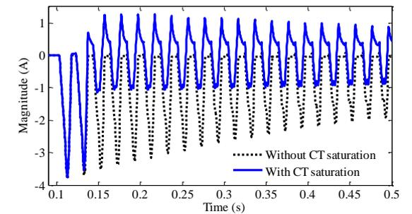
Figure 9. The current of phase A during transformer energization
