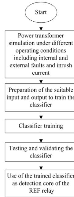
**Figure 12.** The flowchart of the proposed method
