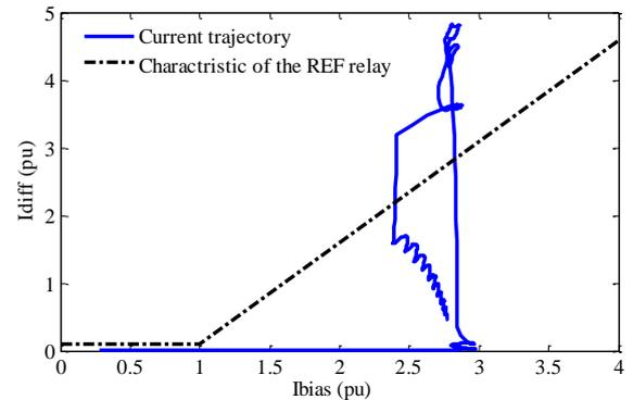
Figure 8. Current trajectory based on the modeled REF relay during external fault with CT saturation
