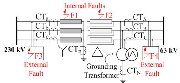
**Figure 2.** The power system under study
