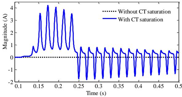
**Figure 10.** Differential current during transformer energization
