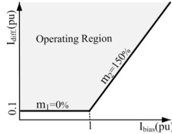
**Figure 1.** The REF relay characteristic with recommended setting [18]
