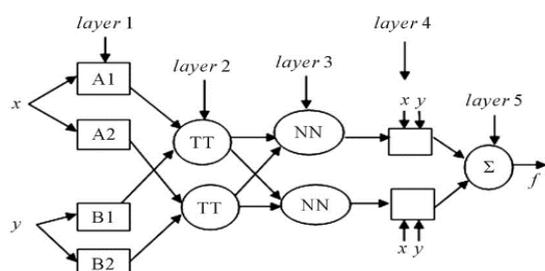
**Figure 2.** Structure of a neuro-fuzzy network
