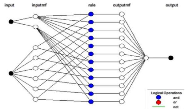
**Figure 4.** Final structure of the ANFIS
