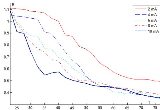
**Figure 3.** Demonstration of the nonlinear characteristics of NTC using real data
