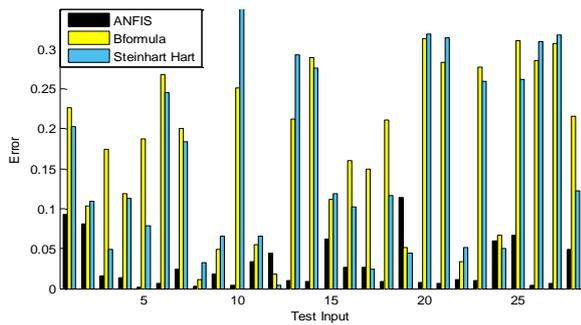
**Figure 7.** Error rates resulting from three methods when applied on the test data
