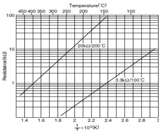
Figure 1. The characteristic diagram of NTC resistor with respect to temperature [13]
