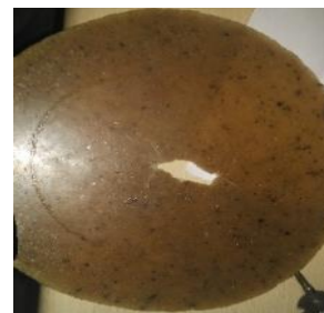
Figure 10. Manufactured Pigmented foil with \text{TiO}_2 and \text{BaSO}_4 embedded in LDPE matrix
