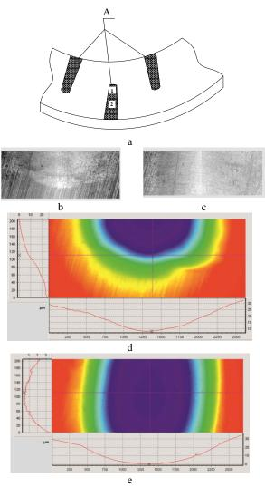
**Figure 3.** Investigation scheme of the inner surface of the outer bearing ring 22316- a, fragments of wear grooves - b, c and corresponding profile charts - d, e; 1,2 – points of surface analysis; A - false brinelling;
