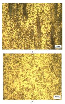
Figure 4. Steel microstructure of bearing 22316
