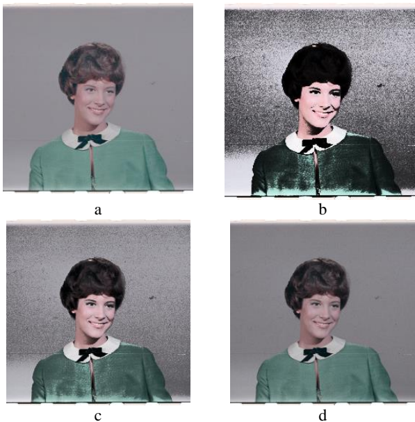
Figure 6. Contrast enhancement result for Girl. (a) Original image, enhanced mages obtained using: (b) HE [8], (c) 2DHE [12], (d) Proposed method
