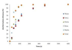
**Figure 4.** Decomposition efficiency of special PCBs and total PCBs by MW (P=500 W, PEG=5 g, NaOH=1 g)
