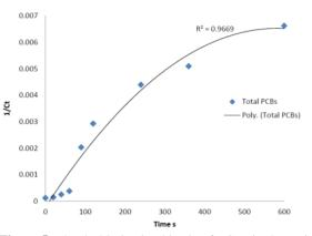
Figure 5. The dechlorination kinetic of PCBs in the optimum amount of variables by MW (PEG=5 g, NaOH= 1 g, P=500W)
