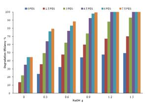
**Figure 2.** PEG influence, in the presence of NaOH, on the dechlorination of PCBs in waste oil by MV power of 500W after 6 min
