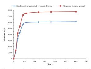
**Figure 7.** Produced chloride ions from dechlorination of PCBs by MW at the end of the process at various times
