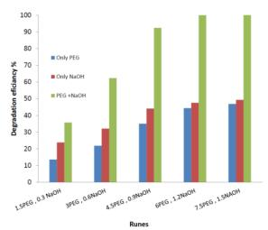
**Figure 3.** NaOH influence, in the presence of PEG, on the dechlorination of PCBs in waste oil under MV power of 500W after 6 min
