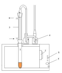
**Figure 1.** Schematic representation of experimental set up; 1. quartz reactor; 2. MV lamp; 3. condenser; 4. vessels containing hexane; 5. switch control; 6. IR-temperature sensor
