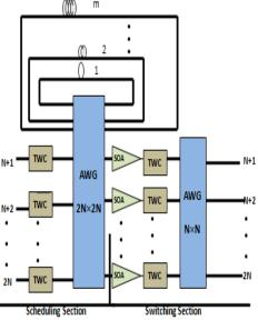
Figure 1. Design of AWG based Switch
