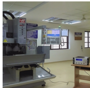
Figure 2. Experimental setup- Machine tool connected with syscon tool dynamometer
