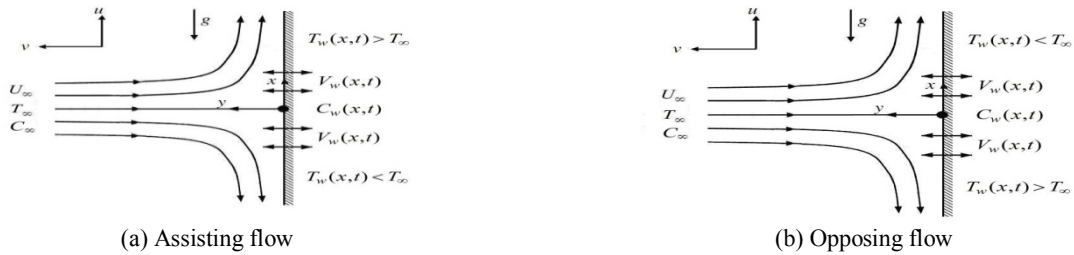
Figure 1. Physical model of two-dimensional stagnation point flow on a vertical surface for prescribed wall temperature case.
