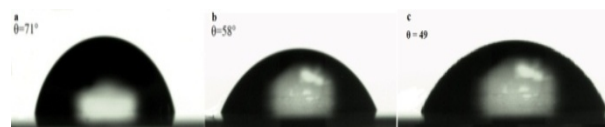
Figure 1. Decreasing in contact angle of a drop of water on PET surface, a) before and b) after treatment, c) after hybrid coating.
