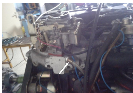
Figure 3. Hydroxy gas entrance to the engine (via an unused entrance of the air intake manifold)
