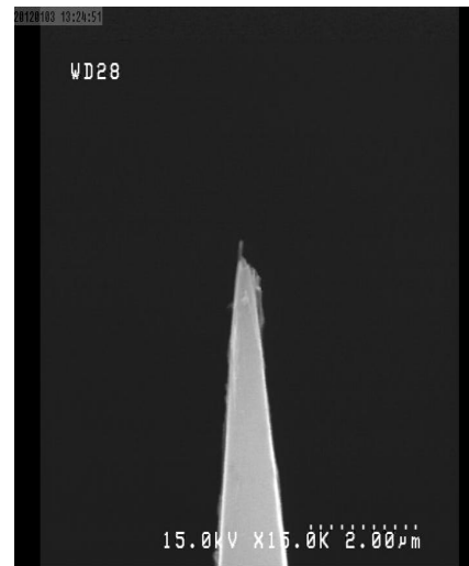
Figure 7. Scanning electron microscopy of CNT tip
