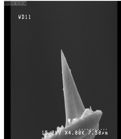
Figure 6. Scanning electron microscopy of conventional Si tip
