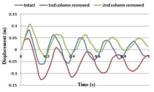
**Figure 14.** Horizontal displacement time history of roof under blast loading (stand-off distance is considered as 30 m)
