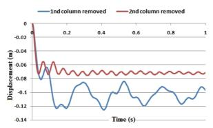
Figure 12. Displacement time history of column removal point under blast loading (stand-off distance is considered as 30 m).
