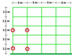
Figure 1. Elevation of model structure and column removal
