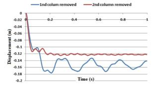
Figure 11. Displacement time history of column removal point under blast loading (stand-off distance is considered as 15 m).
