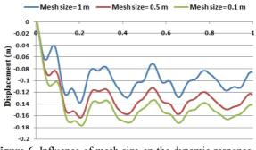
**Figure 6.** Influence of mesh size on the dynamic response of frame under blast loads. (displacement in column removal point, corner column in first story is removed)
