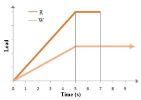
Figure 3. Applied loads for column removal analysis
