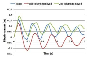
**Figure 13.** Horizontal displacement time history of roof under blast loading (stand-off distance is considered as 15 m)
