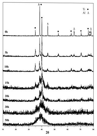
Figure 3. X-ray diffraction patterns of  $Ti_{50}Al_{50}$  elemental powder, mechanically alloyed at several alloying times and with 2wt% Methanol.
