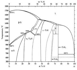
Figure 1. The Ti-Al Diagram [12].
