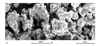
Figure 2. SEM micrographs of pure (a)Ti (b)Al.
