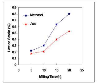
**Figure 7**. The lattice strain of productions of M.A process as a function of alloying time for two PCA.
