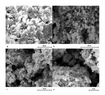
**Figure 9**. SEM micrographs of  $Ti_{50}Al_{50}$  powders mechanically alloyed after (a)5h (b)20h (c)30 and (d)50h with 2%wt stearic acid.
