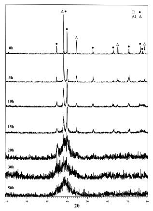
**Figure 4**. X-ray diffraction patterns of  $Ti_{50}Al_{50}$  elemental powder, mechanically alloyed at several alloying times with 2wt% Stearic acid.
