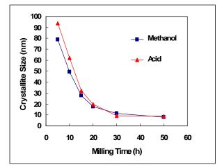
**Figure 6**. The average grain size of productions of M.A process as a function of alloying time for two PCA.
