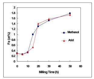
**Figure 11**. The Fe contamination of productions of process as a function of time for two PCA.
