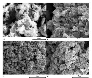
Figure 8. SEM micrographs of  $Ti_{50}Al_{50}$  powders mechanically alloyed after (a)5h (b)20h (c)30 and (d)50h with 2%wt Methanol.
