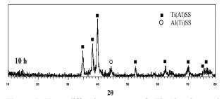
**Figure 5.** X-ray diffraction patterns of  $Ti_{50}Al_{50}$  elemental powder, mechanically alloyed after 10h alloying time and with 2wt% Methanol.
