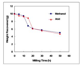
**Figure 10**. The weight recovered of production of process as a function of time for two PCA.
