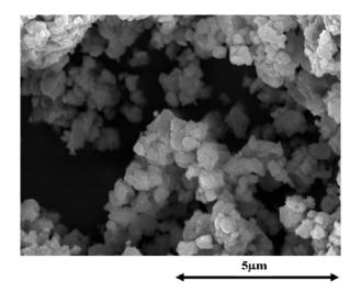
Figure 13. SEM micrographs of mechanically alloyed  $Ti_{50}Al_{50}$  sample after annealed at 900°C for 10min at vacuum oven.
