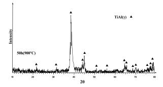
Figure 12. XRD pattern of mechanically alloyed  $Ti_{50}Al_{50}$  after annealed at 900°C for 10min at vacuum oven.
