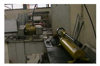
Figure 4. Post-tensioning using hydraulic jack
