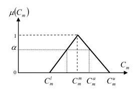
Figure 2. Membership function for a fuzzy capacity of machine type *m*.
