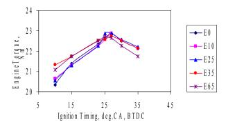
**Figure 3**. Variation of engine torque with ignition timing at the compression ratio of 9:1.
