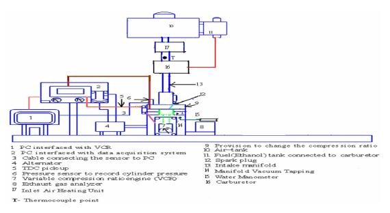
Figure 1. Experimental test rig with necessary instrumentation.
