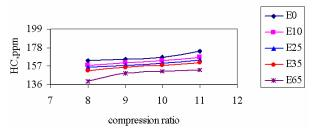
**Figure 13**. Variation of hydrocarbon emissions with compression ratio.
