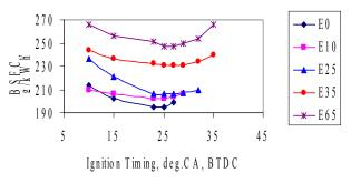
**Figure 4.** Variation of BSFC with ignition timing at the compression ratio of 11:1.
