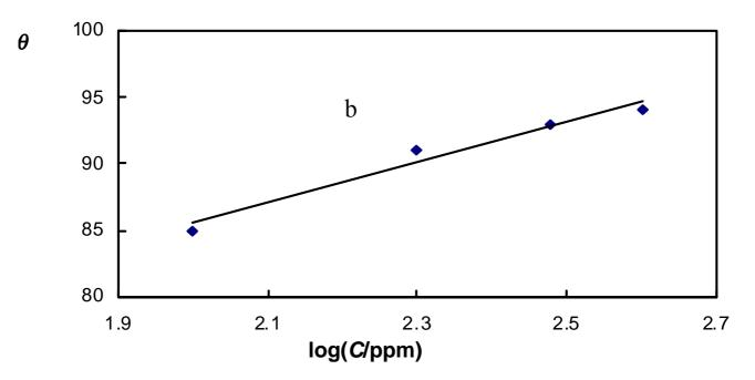
Figure 8b. Adsorption isotherm for BTA and constant concentration of sodium benzoate (200PPM) on mild steel in 0.5 M sulfuric acid.
