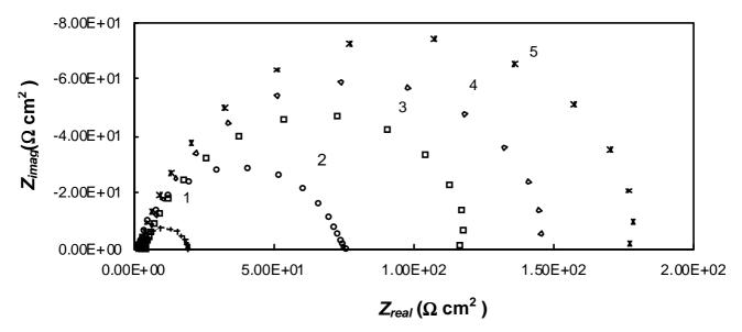
Figure 4. Nyquist plots for mild steel in 0.5 M  $H_2SO_4$  containing different concentration of BTA: 1 - blank, 2 - 100 ppm, 3 - 200 ppm, 4 - 300 ppm and 5 - 400ppm.
