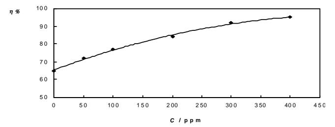
Figure 3. The variation of the inhibition efficiency versus different concentrations of benzoate and constant concentration of BTA (200ppm).
