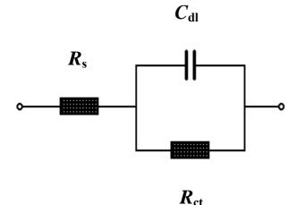
**Figure.7**. Simplified Ershler - Randles circuit ( $R_s$  electrolyte resistance;  $C_{dl}$  double – layer capacitance;  $R_{ct}$  Charge transfer resistance (Equivalent circuit model [R(RQ)].
