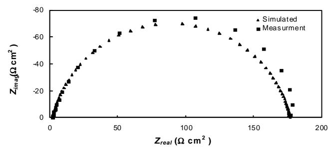
Figure 6. Impedance spectra of mild steel in 0.5 M H<sub>2</sub>SO<sub>4</sub> in the presence of 400PPM BTA (measurement) and fitted results using equivalent circuit model, R(RQ), (Simulated).
