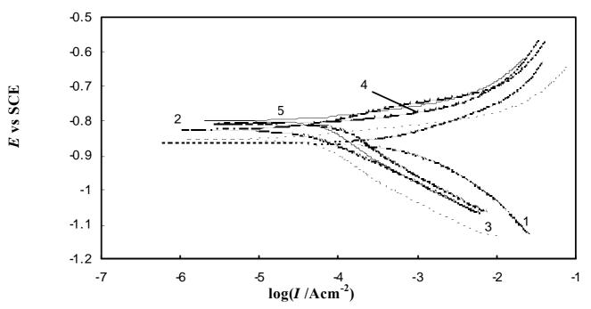
Figure 2. Polarization plots of mild steel in 0.5 M H<sub>2</sub>SO<sub>4</sub> in presence of different concentrations of BTA and constant concentration of sodium benzoate: 1 – blank, 2 – 100 ppm, 3 - 200ppm, 4 – 300 ppm and 5 – 400 ppm.
