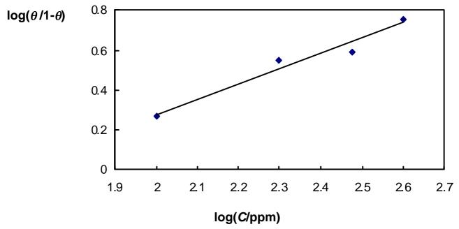
Figure 8a. Adsorption isotherm for BTA on mild steel in 0.5 M sulfuric acid.
