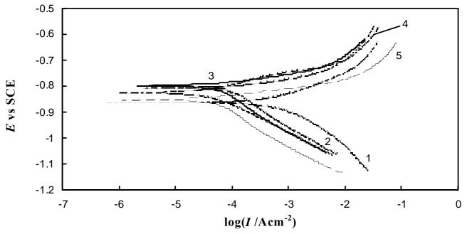
Figure 1. Polarization plots of mild steel in 0.5 M  $H_2SO_4$  in the presence of different concentrations of BTA: 1 - blank, 2 - 100 ppm, 3 - 200 ppm, 4 - 300 ppm and 5 - 400 ppm.
