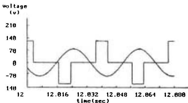
Figure 9. On load input voltage when load applied at t=11 seconds.
