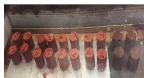
Figure 5. Samples soaked in water for 28 days
