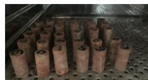
Figure 7. Specimens kept in a water to test under wet condition
