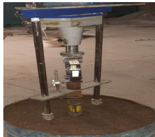
Figure 6. Plate loading tests set
