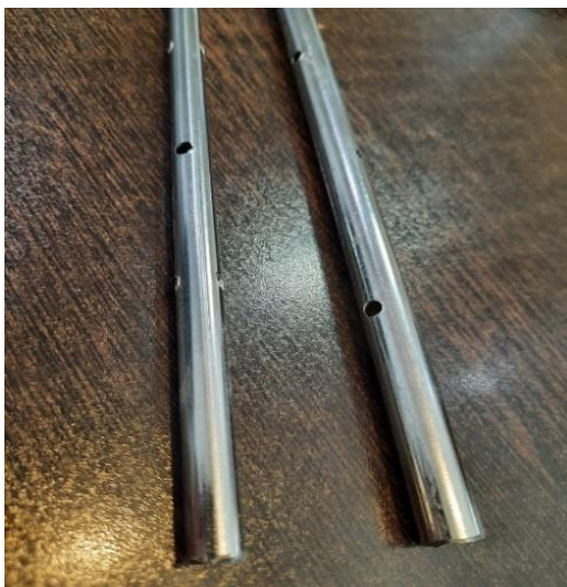
Figure 7. Non-grouted micropiles used in the tests
