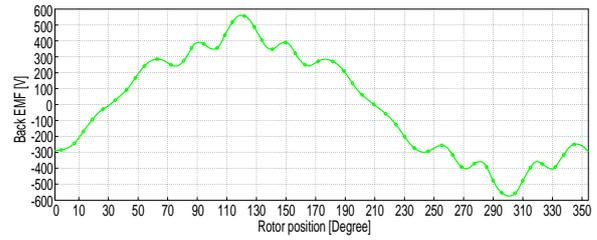
Figure 9. Back EMF waveform without using the skewing technique
