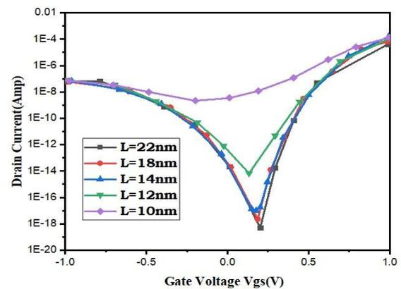
**Figure 6.** Drain current with gate voltage of proposed device at doping concentration  $N_d = 2 \times 10^{18} \text{ cm}^{-3}$
