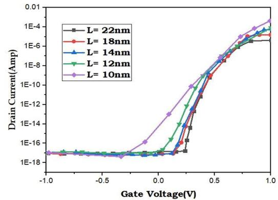
**Figure 5.** Drain current with gate voltage of proposed device at doping concentration  $N_d = 1 \times 10^{18} \text{ cm}^{-3}$
