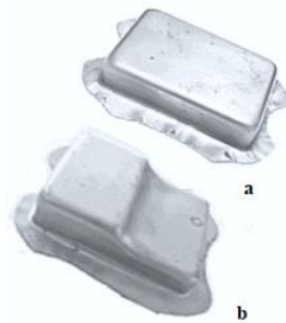
Figure 8. a. Side-step workpiece with a depth of 35 mm and at a pressure of 24 MPa, b. Simple workpiece with a depth of the lower step of 13 mm and at a pressure of 40 MPa, obtained from the experiments
