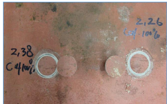
Figure 5. An illustration of AF paint adhesion failure after exposure
