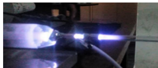
Figure 2. Argon based cold plasma jet using double ring electrode
