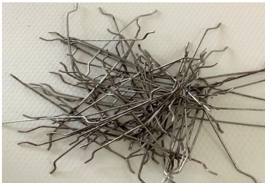
Figure 5. The shape of the fibers with knotted ends used
