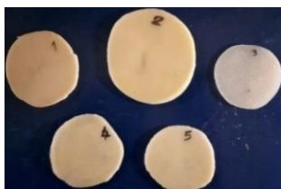
Figure 1. Blended polymer systems onto the calendaring rolls in form of thin layer sheets after hot pressing
