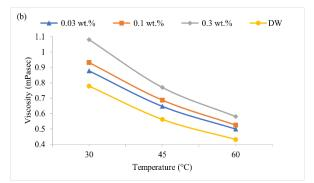
Figure 3(b). Variation of viscosity with temperature
