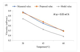
Figure 6(d). Viscosity versus temperature at 0.03 wt.%
