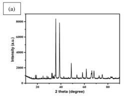
Figure 1(a). XRD pattern of CuO nanoparticles
