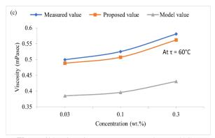
Figure 6(c). Viscosity versus concentration at 60°C
