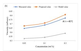
Figure 6 (b). Viscosity versus concentration at 45°C
