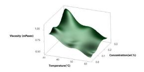
Figure 5 (b). Surface plot showing the relation between the factors and viscosity
