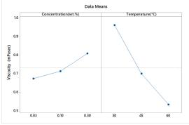
Figure 2. Main effects of the parameters on viscosity
