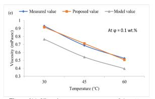
Figure 6(e). Viscosity versus temperature at 0.1 wt.%
