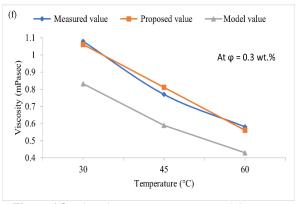
Figure 6(f). Viscosity versus temperature at 0.3 wt.%
