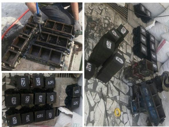
Figure 2. The process of making cubic specimens for compressive tests
