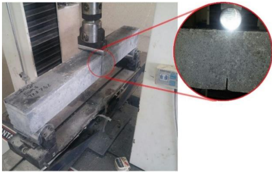
Figure 5. Test setup of bending strength test (Universal testing machine)
