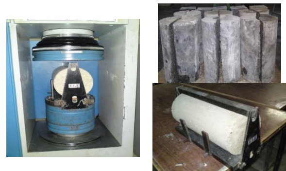
Figure 4. Loading apparatus and specimens for the tensile strength test
