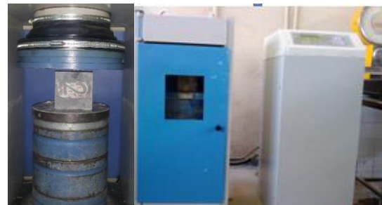
Figure 3. Loading apparatus for the compressive strength test
