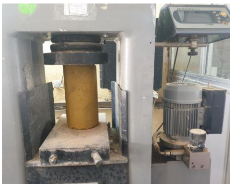
Figure 1. Test of compressive strength
