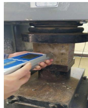
Figure 2. Schmidt hammer test
