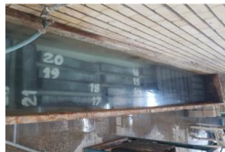
Figure 2. Curing stage of fiber concrete beams
