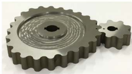
Figure 14. The prototypes of the NCGs pair after manufacture
