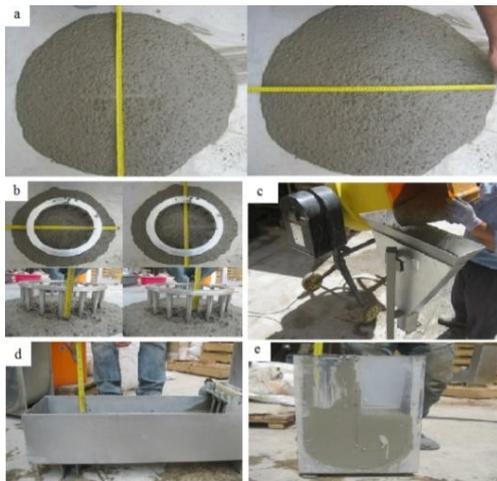
**Figure 4.** Different methods of SCC tests on fresh concrete: a. Slump-flow; b. J-ring; c. V-funnel and V-funnel at T<sub>5minutes</sub>; d. L-box; e. U-box
