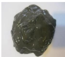
**Figure 3.** Image of micro silica gel used in mix design**TABLE 3.** Chemical and physical properties of MSG
