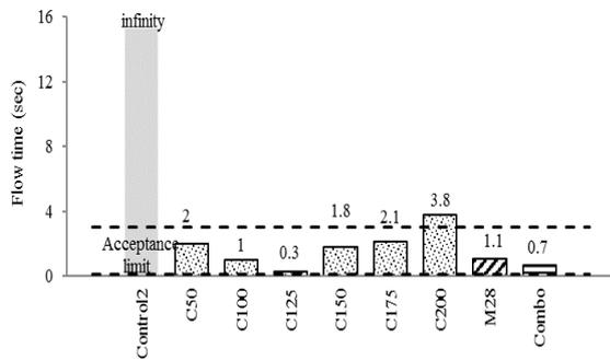
Figure 12. Results of V-funnel test at T<sub>5</sub>minutes
