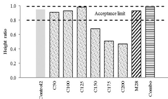
Figure 13. Results of L-Box test
