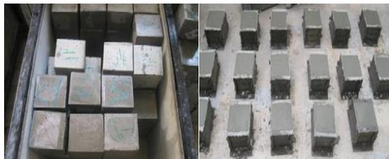
**Figure 5.** Preparation of concrete blocks
