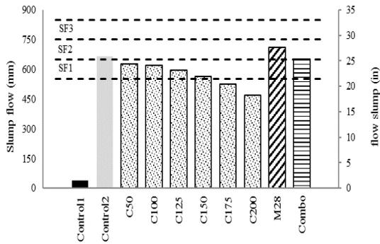
Figure 7. Results of slump flow test
