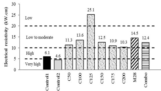
**Figure 18.** Results of electrical resistivity test
