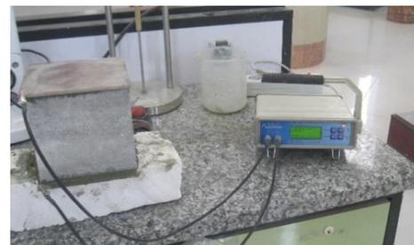
**Figure 6.** Electrical resistivity apparatus
