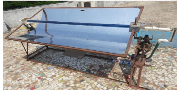
Figure 7. Experimental setup of PTC with two-sided open evacuated tube receiver
