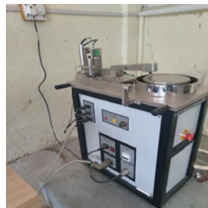
Figure 3. Pin on Disc tribo tester
