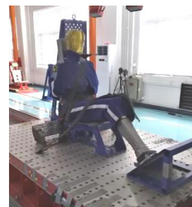
Figure 3. R16 dummy restrained by a 3-point seat belt on the trolley of acceleration type
