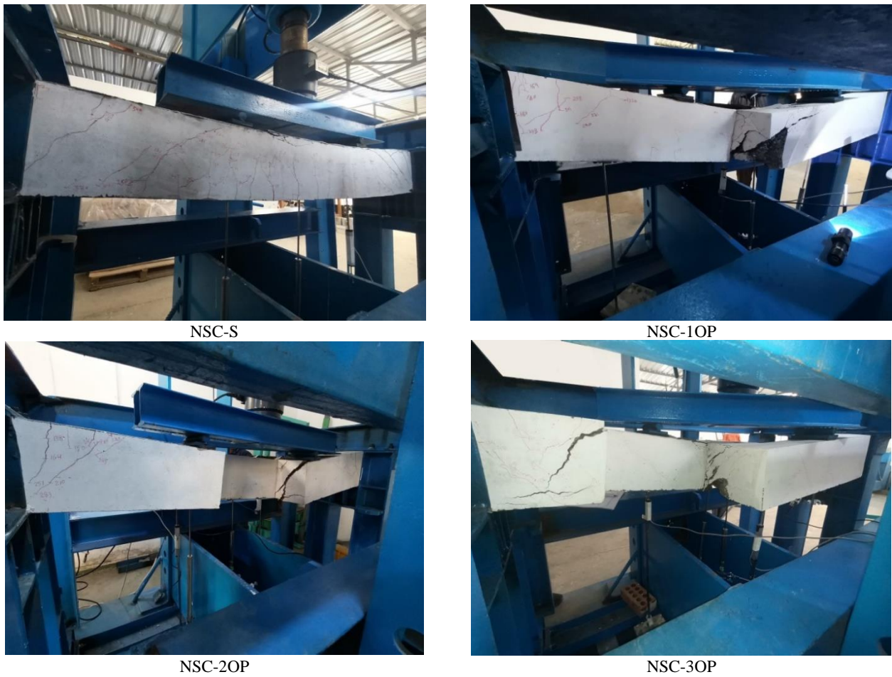
Figure 7. Specimens behavior at the failure load
