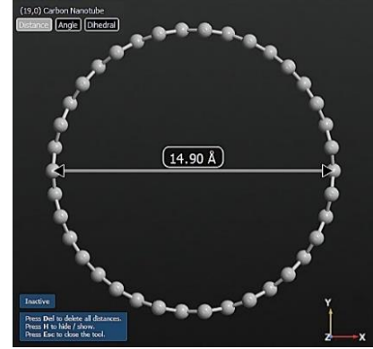
Figure 2. Illustration of diameter calculation for (19, 0) CNT simulated using QuantumWise Atomistix Tool Kit (ATK)
