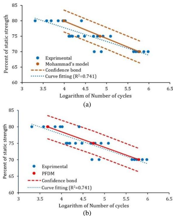
**Figure 8.** Fatigue life simulation and experimental results of  $[90/45/-45/0]_s$  laminate
