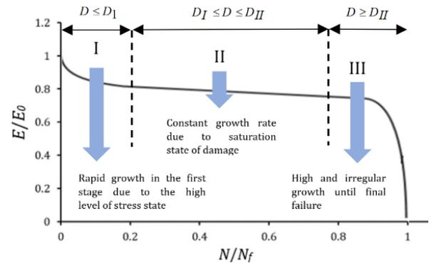
**Figure 1.** Overall stiffness reduction in fatigue loading
