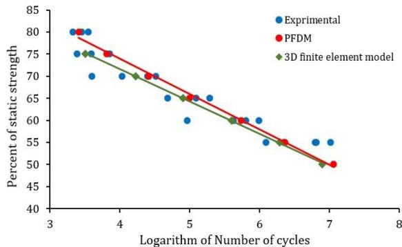
**Figure 6.** Comparison between fatigue life prediction of [30]<sub>16</sub> laminate from different numerical models
