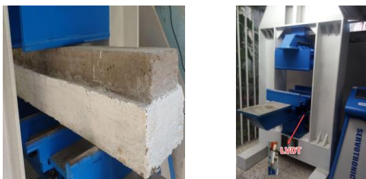
Figure 4. Four-point bending flexural test
