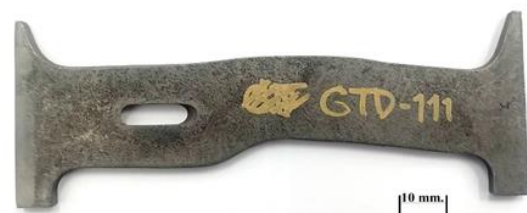
Figure 1. Nickel base superalloys grade GTD111 after long-term service
