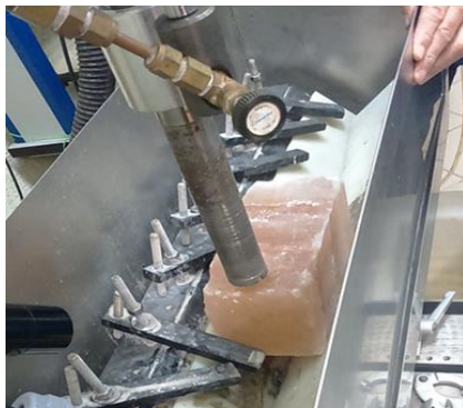
Figure 1. Preparation of NaCl samples using coring machine
