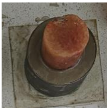
Figure 2. Cylindrical salt sample inside cement
