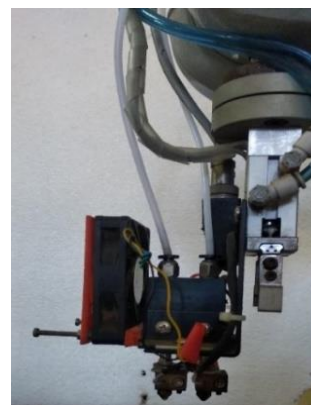
Figure 23. Extruder attached to the robot
