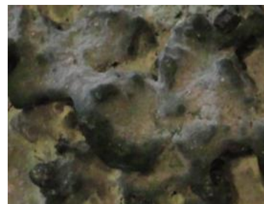
Figure 15. Solid surface formation over the coal ignition area
